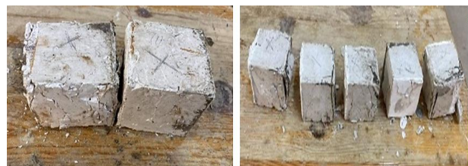
Fig. 16. Specimens of root fibers (left) and remaining fibers on different sieve diameters after failure (right).
