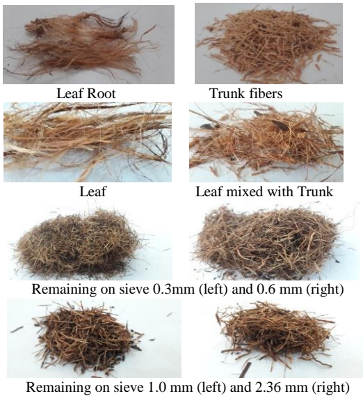
Fig. 3. Fibers extracted from palm tree.
