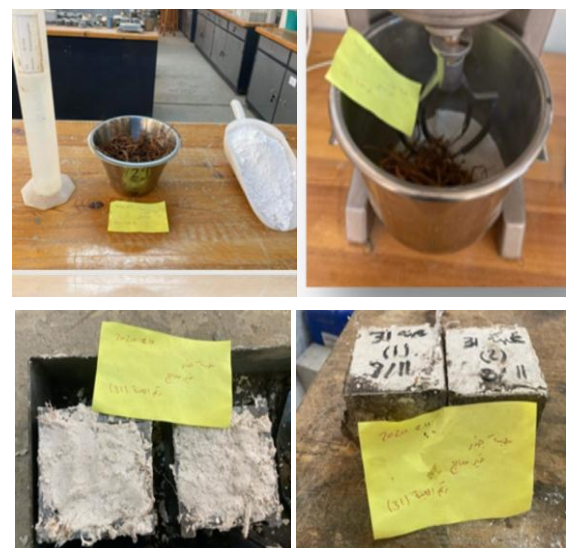
Fig. 4. Preparation specimens of gypsum reinforced by date palm fibers.
