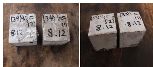
Fig. 5. Specimens of gypsum reinforced by date palm fibers after 24h.
