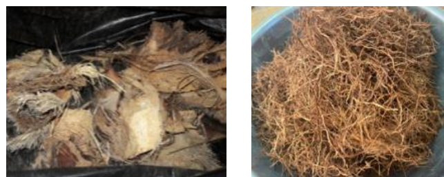
Fig. 2. Palm date tree before (left) and after crumbling (right).
