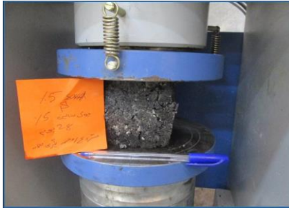
Figure 4: Compressive strength test apparatus (ELE test machine).
