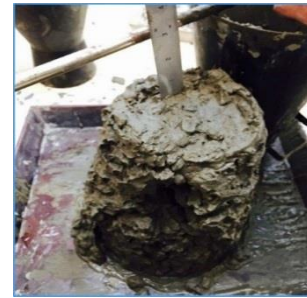
Figure 3. The slump test according to [BS 1881 part 116].
