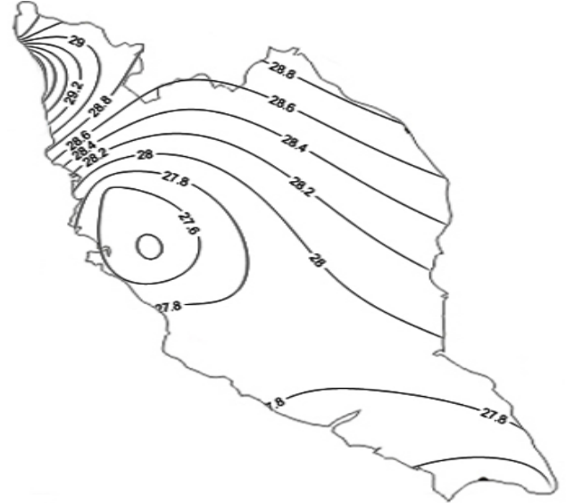
Figure 3. Rain attenuation contour lines in peninsular Malaysia
